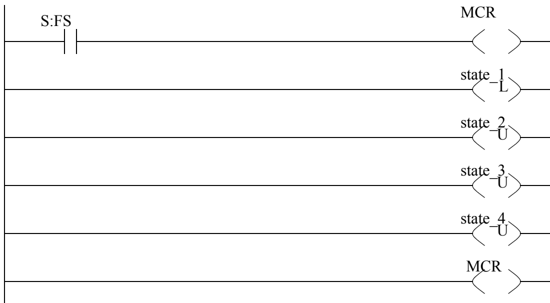
Figure 147 Ladder Logic to Initialize Traffic Light Controller
