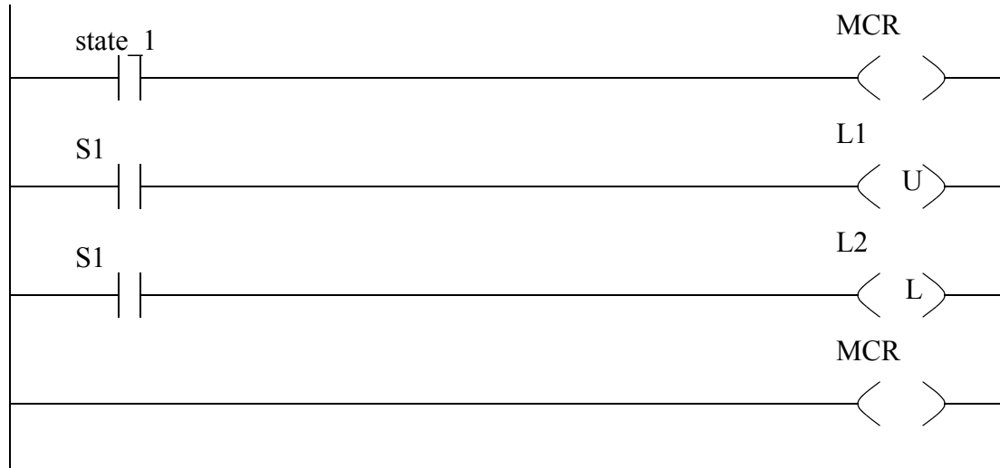
Figure 149 Ladder Logic for First State
